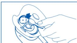
4. Use the supplied cap to close the nebulisation hole located inside the mask (as shown in the picture). The cap should be used only for cleaning purposes.
