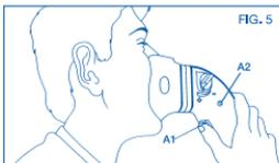
5. Sit comfortably holding nebuliser in a vertical position, bring mask near your face and press the ON/OFF button (A1) for a moment (fig. 5); the nebulizer LED (A2) will show a steady green light and the nebulised medication will start to come out. To increase the effect of the therapy, after inspiration, hold your breath for a second so the drops of inhaled aerosol are able to deposit along the airways. Then slowly breathe out.
