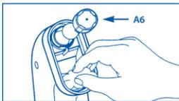
8. Dry the transducer area with a sterile gauze without pressing the transducer. If the transparent cover (A6) looks wet or dirty, take it out and clean it along with its disk.
