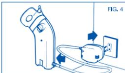
4. Connect the nebuliser to the power mains using the special power unit as indicated (fig. 4). This must be positioned so that it is not difficult to make the disconnection from the mains.
